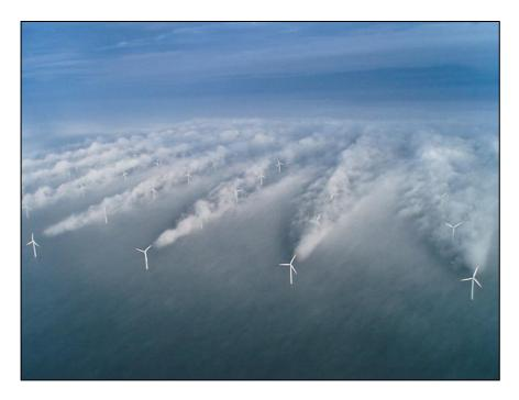
This photo shows rows of wind turbines with moisture illustrating turbulence. The first row of turbines generates turbulence which affects subsequent rows.
