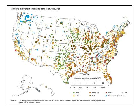
The types of plants range from hydroelectric (most of which are in the Western US) to wind and solar. The one type of plant slowly decreasing in number are coal-fired plants. The green dots are wind projects which are concentrated mostly in the Mid-Western states and Texas.
