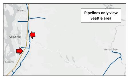
Zooming in on the Seattle area again, we see two major pipelines. After clicking each of the two choices, the **brown colored line** is a **Petroleum Product** Pipeline owned by Enbridge. The **blue line** is a **Natural Gas Interstate** pipeline owned by Northwest Pipeline.
