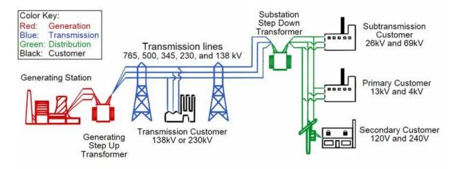
From left to right, the drawing illustrates the generation source (earlier that was the hydroelectric turbine/generation combination) as red. The transformer steps up the voltage for transmission (blue). The step-down transformer reduces the voltage to different levels for different customers vis the distribution systems (green).
