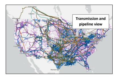
The significance of the EIA database is that you can focus on a specific location. The purple lines are transmission lines and the blue and brown lines pipelines. In the following examples, we will select the Seattle area for additional detail.
